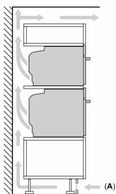
A: Dovod vazduha  $\geq 200 \text{ cm}^2$
