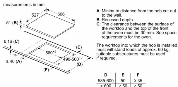
The worktop into which the hob is installed must withstand loads of approx. 60 kg; suitable substructures must be used if required.
