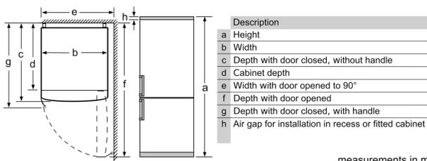
measurements in mm
