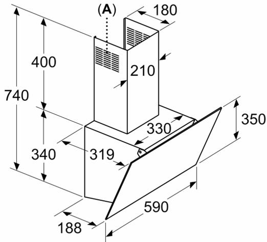
**A:** Air outlet – slots for exhaust air to be mounted facing down
