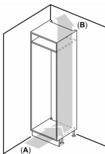
A: Air inlet  $\geq 200 \text{ cm}^2$ ; Ventilation options
