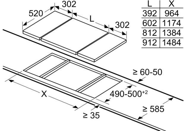
When installing two Domino units right next to a hob, two assembly kits (HZ394301) are required.
