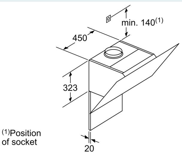
Note the maximum thickness of the back panel.
