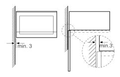
Measurements in mm
