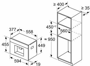
Bean and water containers are removed from the front Recommended installation height 950–1450 mm
