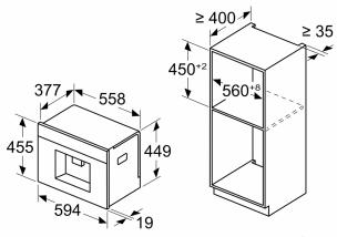
Bean and water containers are removed from the front Recommended installation height 950–1450 mm
