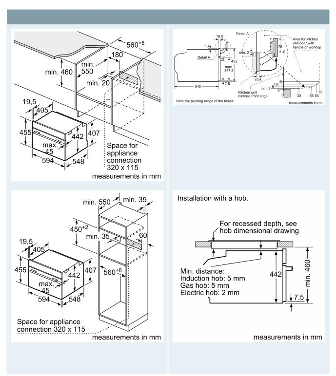
If the compact appliance will be installed underneath a hob, the following worktop thicknesses (including substructure if necessary) must be taken into account.
