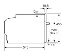
measurements in mm
