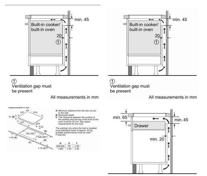
Measurements in mm
