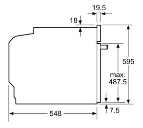
measurements in mm
