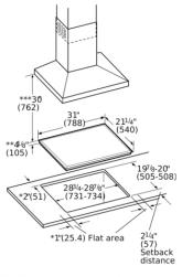
\*Minimum distance from cutout to the wa \*\*Installed depth includes a required 1° (26mm) air gap \*\*Minimum distance between the hob and lower edge of the exhaust hood
