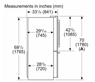
A: Add 1/4" (6 mm) with front leveling feet fully extended
