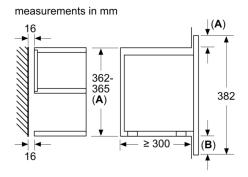
A: Overhang at top: Recess 362: 6 mm Recess 365: 3 mm B: Overhang at bottom: 14 mm
