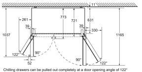
nilling drawers can be pulled out completely at a door opening angle of 122° measurements in mm
