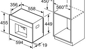
Bean and water containers are removed from the front. Recommended installation height 95-145 cm. measurements in mm
