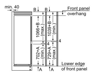
measurements in mm Recommended gap dimensions for flat hinges
