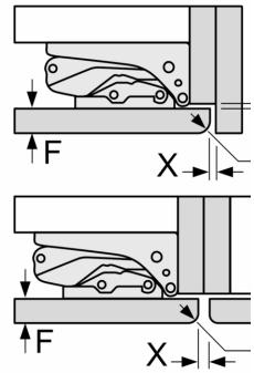
The gap dimensions in the table must be observed to ensure that any parts of the appliance do not collide with anything and to avoid causing damage.
