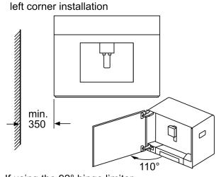
If using the 92° hinge limiter (spare part no. 00636455), the minimum distance to the wall is only 100 mm. measurements in mm
