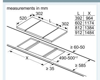
When installing two Domino units right next to a hob, two assembly kits (HZ394301) are required.
