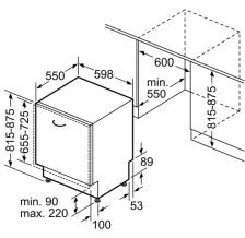
measurements in mm
