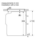
A: Recessed depth 29-50 mm. See hob dimensional drawing. B: Min. distance: Induction hob: 5 mm Gas hob: 5 mm Electric hob: 2 mm
