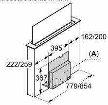
A: Access to the entire cover must be ensured even after installation.
