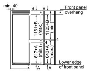
Recommended gap dimensions for flat hinges X
