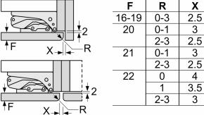
The specified unit door dimensions are valid for a door gap of 4 mm.
