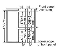
The specified unit door dimensions are valid for a door gap of 4 mm. If a different gap width is used (max. 14 mm), the dimensions must be adjusted.
