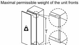
Fitted kitchen unit doors that exceed the permissible weight may cause damage and result in functional impairment of the hinges.
