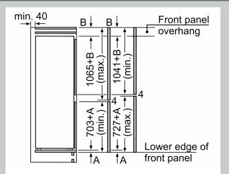
The specified unit door dimensions are valid for a door gap of 4 mm. measurements in mm measurements in mm Recommended gap dimensions for flat hinges
