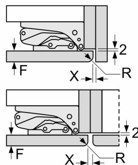
The gap dimensions recommended in the table must be adhered to in order to ensure that appliance doors do not collide with anything when they are opened, and to avoid causing damage to kitchen units.
