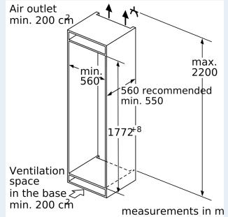
measurements in mm Recommended gap dimensions for flat hinges
