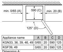
Dimension A: In models with vertical integrated handles, in order to open easily, a minimum distance of 65 mm is needed.
