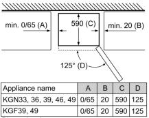
Dimension A: In models with vertical integrated handles, in order to open easily, a minimum distance of 65 mm is needed.
