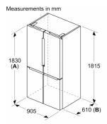
A: Front is adjustable 1830–1847 mm, with front levelling feet fully extended
