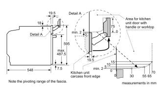
measurements in mm
