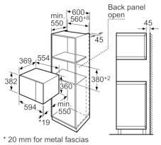
measurements in mm
