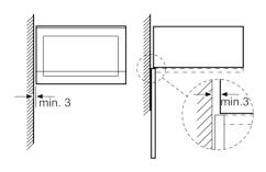
Measurements in mm
