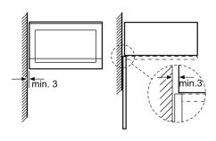
Measurements in mm
