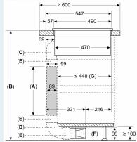
A: Tube length B: Kitchen height C: 90° S-size bow D: 90° L-size bow E: Connector sleeve F: Diffusor G: Shortened Drawer
