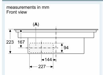
measurements in mm Front view – unit cut-out for unducted recirculation
