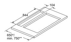
Only install one side of the appliance at least 50 mm from a high-sided unit or a wall.
