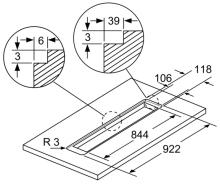
For flush installation in stone and granite work surfaces
