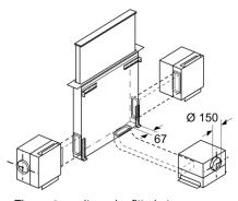
The motor unit can be fitted at a maximum distance of three metres from the appliance. (Special accessory required)
