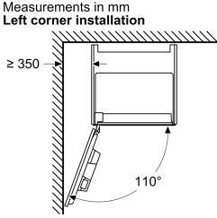
If using the 92° hinge limiter, the min. distance to the wall is only 100  $\,\rm mm$
