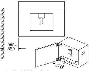
If using the 92° hinge limiter (spare part no. 00636455), the minimum distance to the wall is only 100 mm. measurements in mm
