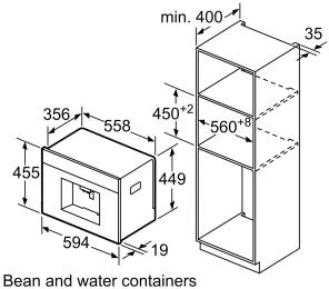
are removed from the front. Recommended installation height 95-145 cm. measurements in mm
