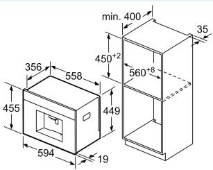
are removed from the front. Recommended installation height 95-145 cm. measurements in mm
