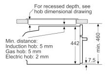
measurements in mm
