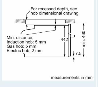
If the compact appliance will be installed underneath a hob, the following worktop thicknesses (including substructure if necessary) must be taken into acccount.
