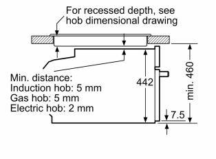
measurements in mm
