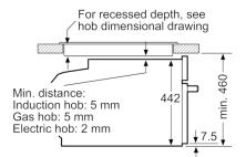
measurements in mm
