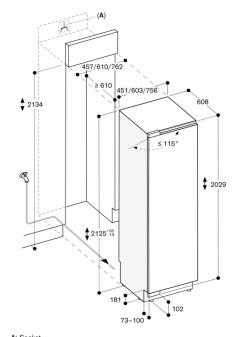
**A:** Socket Maximum door panel dimensions are based on a clearance of 3 mm
