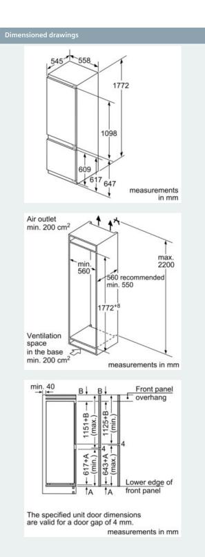
measurements in mm Recommended gap dimensions for flat hinges
