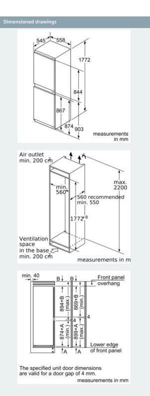
measurements in mm Recommended gap dimensions for flat hinges
