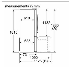
A: Front is adjustable from 1830 to 1847, with front levelling feet fully extended
